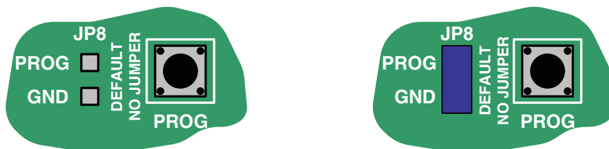
a) No Jumper: FPGA Operational (default)
