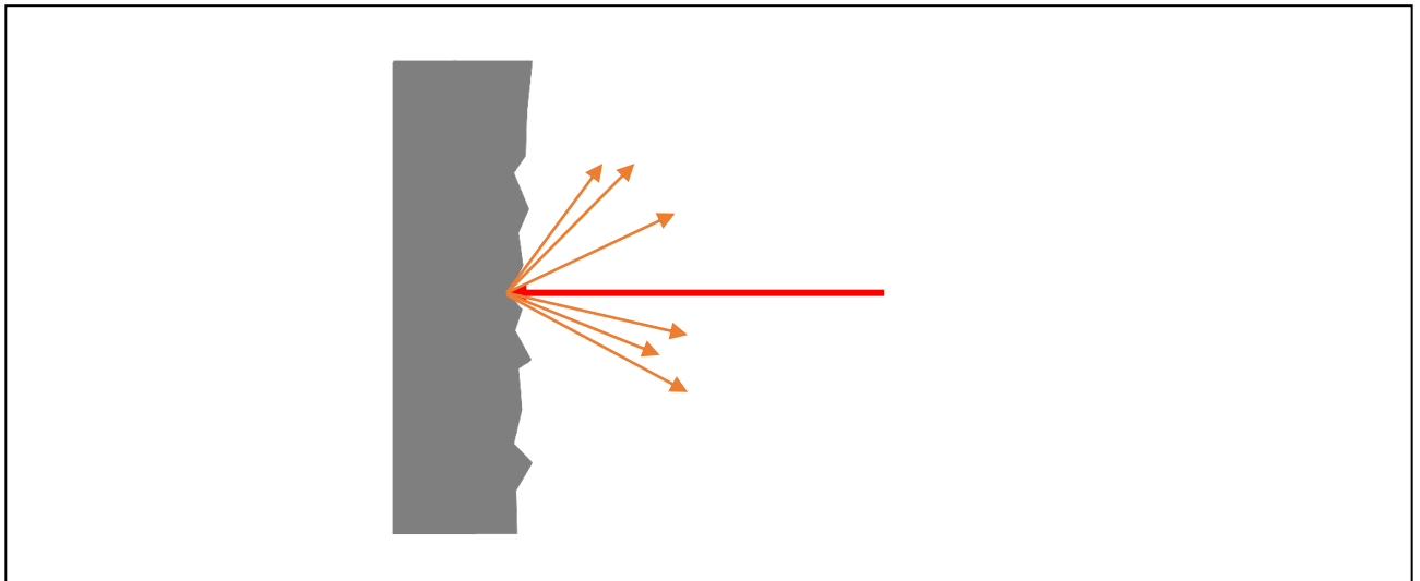
Figure 19 Reflection of the laser beam at the surface of an object
