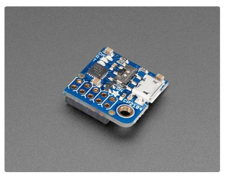
Here's another super handy add-on for your Raspberry Pi computer, perfect for 'headless' setups! The <u>PiUART</u> (https://adafru.it/zib) adds a MicroUSB to serial connection so you can use any serial port software to connect to the Pi's console. It plugs in and is fast and easy to add whenever you need to connect to your Pi. Two LEDs connect to RX and TX on the serial converter chip so you get blinking whenever data is sent or received.
