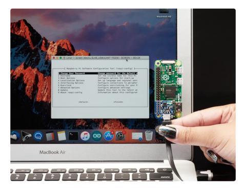
We had some space left over, so the PiUART also comes with an on-off switch with a 4 Amp transistor. You can power your Pi through the microUSB port and then use the switch whenever you want to cut power, without having to unplug the cable. Low-power usage Pi's like the Pi Zero and A+ can thus be powered and controlled from a single cable connected to your computer.
