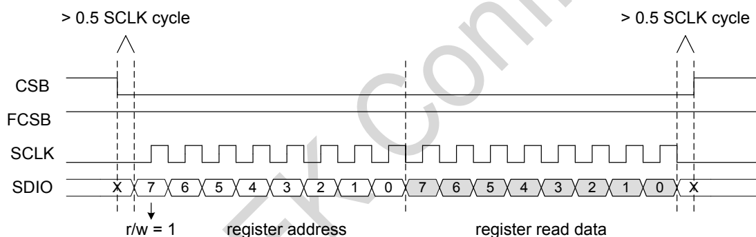
Figure 9. SPI read register timing
