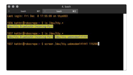
Press enter to run the command. It will open in the same window. If no code is running, the window will be blank. Otherwise, you'll see the output of your code.
