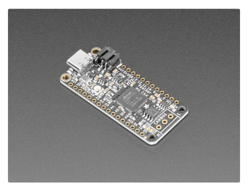
At the end of the board we have placed a CAN transceiver chip as well as a 5V converter to generate 5V power to the transceiver even when running on battery. The two CAN signal lines and ground reference signal are available on a 3-pin 3.5mm terminal block. The chip and booster can be put to sleep for power saving. The built in CAN can read or write packets and has support in both Arduino and CircuitPython.
