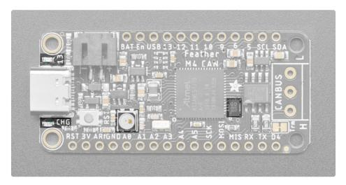
**NeoPixel LED -** connected to pin #8 in Arduino, so just use our NeoPixel library (https://adafru.it/dhw) and set it up as a single-LED strand on pin 8. In CircuitPython, the NeoPixel is board.NEOPIXEL and the library for it is <u>here</u> (https://adafru.it/wby) and in <u>the bundle</u> (https://adafru.it/uap).
