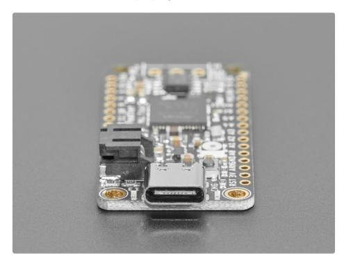
**Easy reprogramming**: the Feather M4 CAN comes pre-loaded with the <u>UF2</u> <u>bootloader</u> (https://adafru.it/vQd), which looks like a USB storage key. Simply drag firmware on to program, no special tools or drivers needed! It can be used to load up CircuitPython or Arduino IDE (it is bossacompatible)
