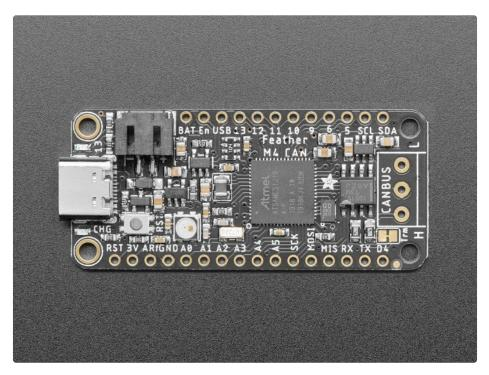
One of our favorite Feathers, the Feather M4 Express, gets a glow-up here with an upgrade to the SAME51 chipset which has built-in CAN bus support! Like its SAMD51 cousin, the **ATSAME51J19** comes with a **120MHz Cortex M4** with floating point support and **512KB Flash and 192KB RAM**. Your code will zig and zag and zoom, and with a bunch of extra peripherals for support, this will for sure be your favorite new chipset for CAN interfacing projects.
