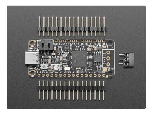
The Feather M4 Can Express also comes with a Mini NeoPixel and 2 MB SPI Flash storage. You can use the SPI Flash storage like a very tiny hard drive. When used in CircuitPython, the 2 MB flash acts as storage for all your scripts, libraries and files. When used in Arduino, you can read/write files to it, like a little datalogger or SD card, and then with our helper program, access the files over USB.
