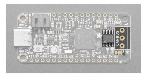
The SAMDE51 has built in hardware CAN bus support, but you still need a transceiver.
