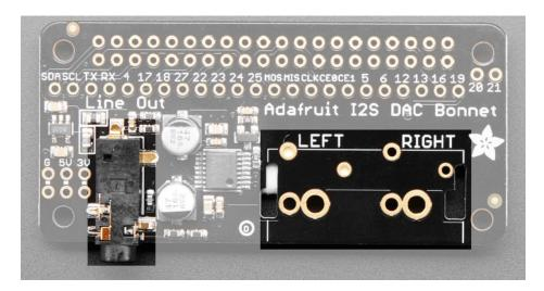
There's also a breakout slot for soldering in dual/stereo RCA jacks, not included with the bonnet.
