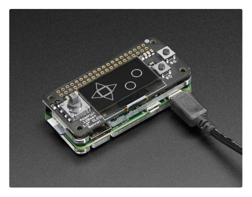
These displays are small, only about 1.3" diagonal, but very readable due to the high contrast of an OLED display. This screen is made of 128x64 individual white OLED pixels and because the display makes its own light, no backlight is required. This reduces the power required to run the OLED and is why the display has such high contrast; we really like this miniature display for its crispness!
