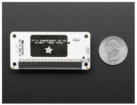
Best of all, this Bonnet is fully assembled - no soldering at all is required. You may need to solder headers onto your Pi Zero (or use press-fit headers) but once that's done you're ready to rock. In theory you could also use this with a Pi A+ or B+/2/3 but it wouldn't be very hand-held
