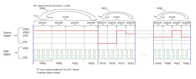
Figure 6-5 : Gate waveform and Programmable Source and VCOM waveform illustration
