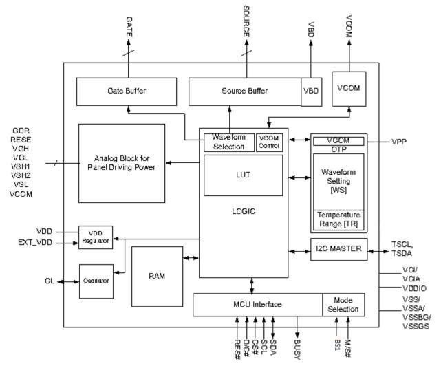
Figure 4-1 : SSD1675 Block Diagram
