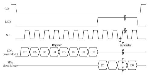
Figure 6-2 : Read procedure in 4-wire SPI mode
