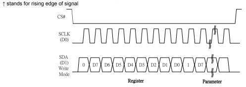
Figure 6-3 : Write procedure in 3-wire SPI
