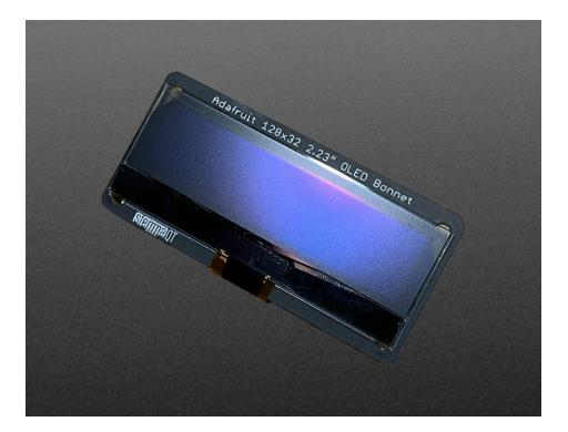
Compared to our similar PiOLED display (https://adafru.it/wVd), this OLED has the same resolution but is much larger, so it can be read from across the room. This screen is made of 128x32 individual white OLED pixels and because the display makes its own light, no backlight is required. This reduces the power required to run the OLED and is why the display has such high contrast; we really like OLED displays for their crispness!
