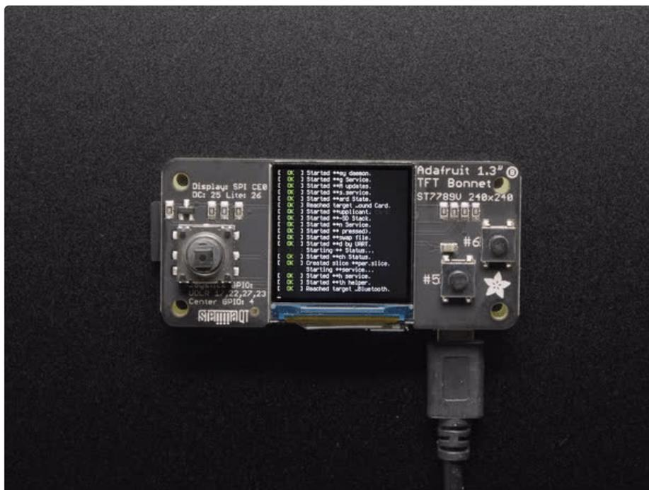
We don't recommend using the 240x240 display for GUI/PIXEL desktop, this is only for text console usage. The display is waaay too small for a desktop
