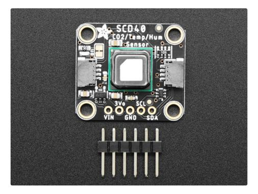
The SCD-40 and SCD-41 are photoacoustic 'true' CO2 sensors that will tell you the CO2 PPM (parts-permillion) composition of ambient air. <u>Unlike the SGP30</u>, this sensor isn't approximating it from VOC gas concentration (https://adafru.it/PF7) - they really are measuring the CO2 concentration! That means they're bigger and more expensive, but they are the real thing. Perfect for environmental sensing, scientific experiments, air quality and ventilation studies, and more.
