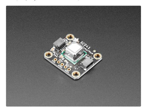
Compared to the illustrious SCD-30 (https://adafru.it/QfK), this sensor uses a different measurement technique, which allows it to be much smaller. The overall data quality should be very similar, however. Like the SCD-30, this sensor has data read over I2C, so it works very nicely with just about any microcontroller or microcomputer. There's both Arduino and Python/CircuitPython code so you can get started in a jiffy.
