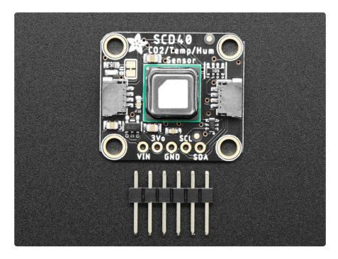
The SCD-40 and SCD-41 are photoacoustic 'true' CO2 sensors that will tell you the CO2 PPM (parts-per-million) composition of ambient air. Unlike the SGP30, this sensor isn't approximating it from VOC gas concentration (https://adafru.it/PF7) - they really are measuring the CO2 concentration! That means they're bigger and more expensive, but they are the real thing. Perfect for environmental sensing, scientific experiments, air quality and ventilation studies, and more.
