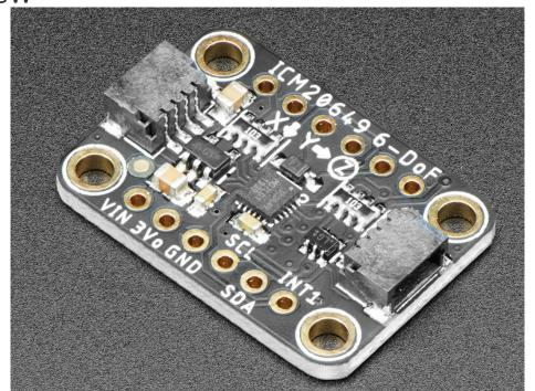
Most accelerometers have a similar range of measurements that they can make: often around 2G - 16G. Similarly most gyros can measure in the range of 250 degree/s to 2000 degrees/s. That's enough for many situations, however there are many situations where it's not quite enough. When measuring things like a golf swing, soccer ball kick or perhaps a fancy racing car, you need a bit more performance out of your motion sensor.
