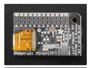
Both the 1.3" and 1.14" versions of the Mini PiTFT have the same 2x12 connector and pinouts.
