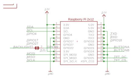
The mini PiTFT connects to the 'top' 2x12 headers on the Pi's 2x20 header connection. It uses the following pins:
