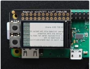
If you ever get a display like this, it means your kernel changed - either due to an upgrade/update or because you switched Pi boards. The solution is to simply re-run the scripts above!
