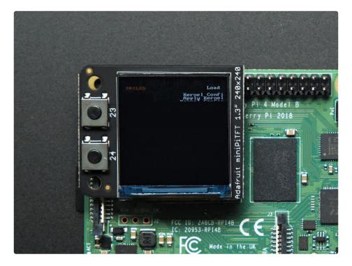
The Adafruit Mini PiTFT - 240x240 Color TFT Add-on for Raspberry Pi is a bit larger, 1.3" diagonal and
