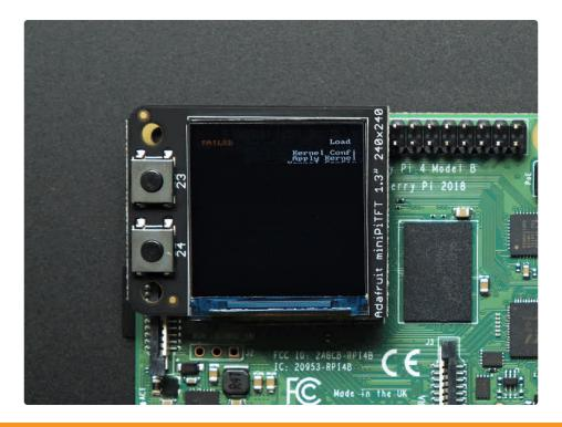
We don't recommend using the 240x240 display for GUI/PIXEL desktop, this is only for text console usage. The display is waaay too small for a desktop
