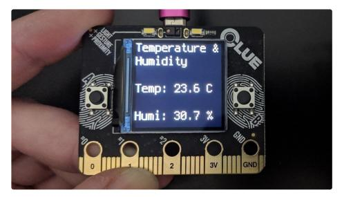
The Adafruit CLUE has a temperature and humidity sensor that reads the temperature in degrees Celsius and the relative humidity in percent. To learn more about relative humidity, check <a href="Wikipedia">Wikipedia</a> (https://adafru.it/CxM).
