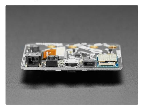
The CLUE is designed for projects that use a ton of sensors - and they're all built in! So you can start exploring your world, measuring, logging and learning. You can transmit data over Bluetooth to a computer or mobile device for data plotting and logging, or save it to the built in storage.
