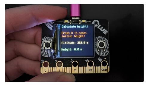
The Adafruit CLUE has a barometric pressure sensor that uses the pressure readings to calculate altitude. For more information on how this works, check out Wikipedia (https://adafru.it/J2e).
