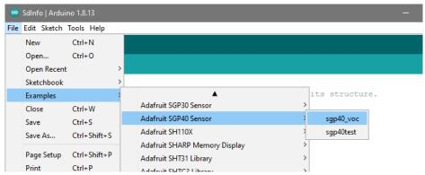
After opening the demo file, upload to your Arduino wired up to the sensor. Once you upload the code, you will see the **raw measurement** and **VOC Index** values being printed when you open the Serial Monitor (**Tools->Serial Monitor**) at **115200 baud**, similar to this:
