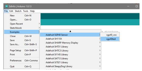
After opening the demo file, upload to your Arduino wired up to the sensor. Once you upload the code, you will see the **Raw measurement** values being printed when you open the Serial Monitor (**Tools->Serial Monitor**) at **115200 baud**, similar to this:
