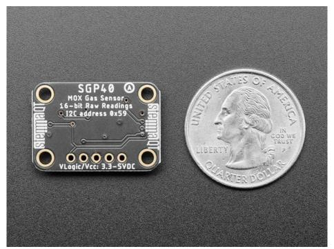
The SGP40 has a 'standard' hot-plate MOX sensor, as well as a small microcontroller that controls power to the plate, reads the analog voltage and provides an I2C interface to read from. Unlike the CCS811, this
