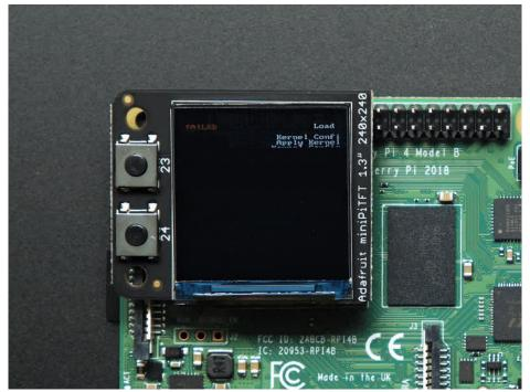
The Adafruit Mini PiTFT - 240x240 Color TFT Add-on for Raspberry Pi is a bit larger, 1.3" diagonal and has 240x240 pixels instead of 240x135
