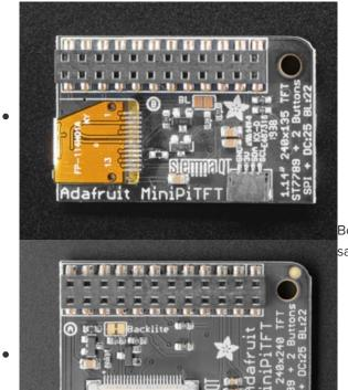
Both the 1.3" and 1.14" versions of the Mini PiTFT have the same 2x12 connector and pinouts.
