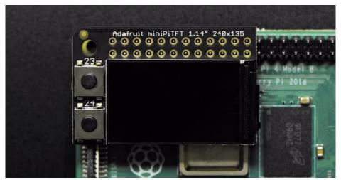
The Adafruit Mini PiTFT - 135x240 Color TFT Add-on for Raspberry Pi is your little TFT pal, ready to snap onto any and all Raspberry Pi computers, to give you a little display. The Mini PiTFT comes with a full color 240x135 pixel IPS display with great visibility at all angles. The TFT uses only the SPI port so its very fast, and we leave plenty of pins remaining available for buttons, LEDs, sensors, etc. It's also nice and compact so it will fit into any case.
