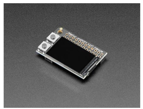
These display are super small, only about 1.14" or 1.3" diagonal, but since they are IPS displays, both are very readable with high contrast and visibility. We had a little space on the PCB so we give you two tactile buttons on GPIO pins so you can create a simple user interface. On the bottom we have a Qwiic/STEMMA QT connector for I2C sensors and device so you can plug and play any of our STEMMA QT devices (https://adafru.it/GfR).
