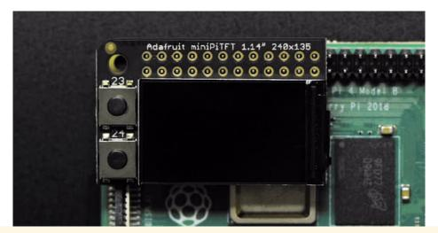
You will not get a GUI/LXDE display, this is only for text console usage. The display is waaay too small for LXDE
