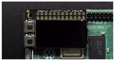
Attach power to the Pi and re-log in. The PiTFT should be lit but nothing on the screen.
