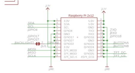
The mini PiTFT connects to the 'top' 2x12 headers on the Pi's 2x20 header connection. It uses the following pins:
