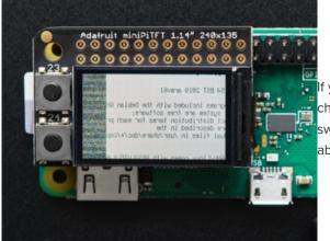
If you ever get a display like this, it means your kernel changed - either due to an upgrade/update or because you switched Pi boards. The solution is to simply re-run the scripts above!
