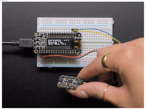
The MPU-6050 is a popular six DoF accelerometer and gyroscope (gyro) that has all the info you need on how things are shakin' and spinnin'. With six axes of sensing and 16-bit measurements, you'll have everything you need to give your robot friend a sense of balance, using the MPU-6050 as its inner ear.
