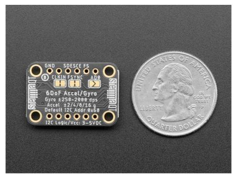
As with all Adafruit breakouts, we've done the work to make the MPU-6050 super easy to use. We've put it on a breakout board with the required support circuitry and connectors to make it easy to work with. Anc of course we've added SparkFun Qwiic (https://adafru.it/Fpw) compatible STEMMA
