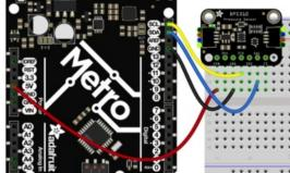
The final results should resemble the illustration above, showing an Adafruit Metro development board.
