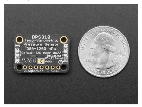
You can use this sensor with either I2C or SPI, so it's easy to integrate into projects. It also has a temperature sensor built in, with  $\pm$  0.5°C accuracy. For the lowest noise readings, set it up to take multiple measurements and perform a low-pass filter, that capability is built in! You can use it from 300 to 1200 hPa and in ambient temperature ranges from -40 to 85 °C.
