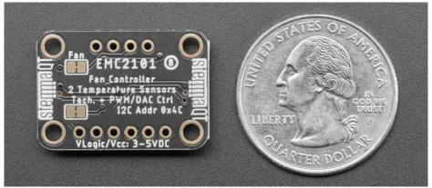
This neat little chip can easily be used to help provide cooling or ventilation to your next project. You might even be able to use it to help quiet down an existing project or hack a noisy piece of electronics that has a loud fan. By allowing you to run a fan at slower speeds when cooling needs are moderate, the EMC2101 can help ease the vibration noise caused by fans running at full speed.
