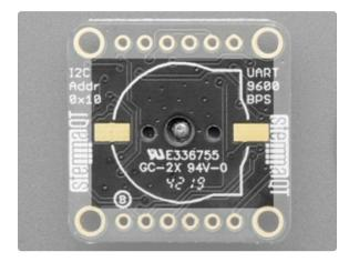
The back has a footprint for an **optional coin cell battery**. The board ships with a CR1220 coin cell holder that can be soldered onto the back. CR1220 battery not included.
