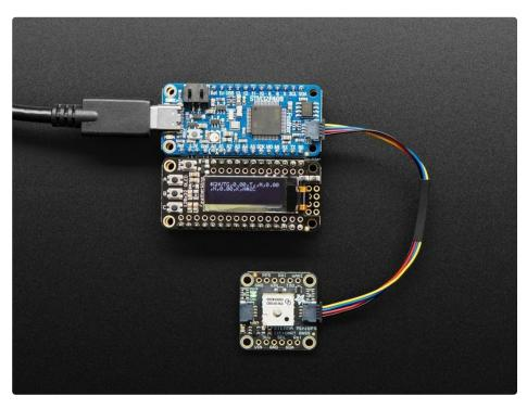
This miniature GPS breakout is only 1" x 1" ( $\sim$  25mm x 25mm) but houses a complete GPS/GNSS solution with both I2C and UART interfaces. There's even an antenna on top so it's plug and play!
