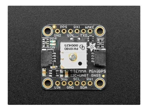
The breakout is built around the MTK3333 chipset, a reliable, high-quality GPS module that can handle up to 33 simultaneous tracking channels, has an excellent high-sensitivity receiver (-165 dBm tracking!), and a built in antenna. It can do up to 10 location updates a second for high speed, high sensitivity logging or tracking. Power usage is incredibly low, only 30 mA during navigation.
