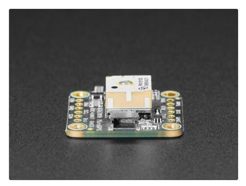
Best of all, we added all the extra goodies you could ever want: a ultra-low dropout 3.3V regulator so you can power it with 3.3-5VDC in, 5V level safe inputs on UART and I2C, a footprint for optional CR1220 coin cell to keep the RTC running and allow warm starts, a green power LED and a tiny red PPS LED. The LED
