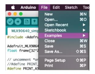
Go to File > Examples > Adafruit MLS90640 > MLX90640\_arcadacam to open the ArcadaCam Arduino thermal camera example, and then load it onto your PyBadge or PyGamer.
