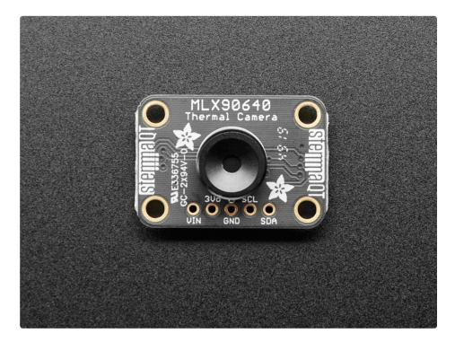
You can now add affordable heat-vision to your project with an Adafruit MLX90640 Thermal Camera Breakout. This sensor contains a 24x32 array of IR thermal sensors. When connected to your microcontroller (or Raspberry Pi) it will return an array of 768 individual infrared temperature readings over I2C. It's like those fancy thermal cameras, but compact and simple enough for easy integration.
