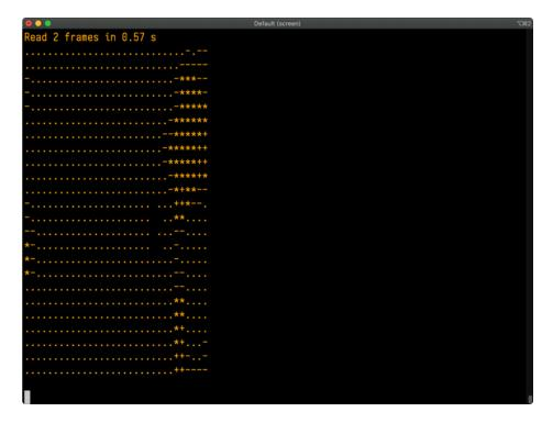
If you change the values for the variables at the top of the program, you can switch from printing out an ASCII image to printing out the temperatures in a grid. Change PRINT\_TEMPERATURES to True and
