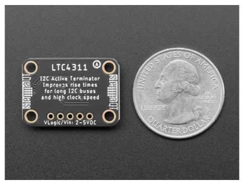
Runs with any bus voltage, from 1.6V to 5.5V and up to 400 KHz SCL speed, with cables up to 4000pF. No special firmware, software, or configuration required. Simply plug the power, ground, SCL and SDA connectors into your bus and watch as your rise times magically turn sawtooths into square waves.
