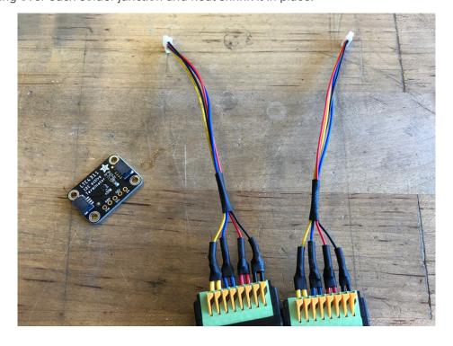
Now, you can plug in any length (up to about 100 feet / 30 meters seems to work well) of Ethernet cable, and then plug the STEMMA QT cables into your sensor on one end and the LTC4311 terminator on the other. Connect the LTC4311's other connector to your microcontroller and you're ready to go!
