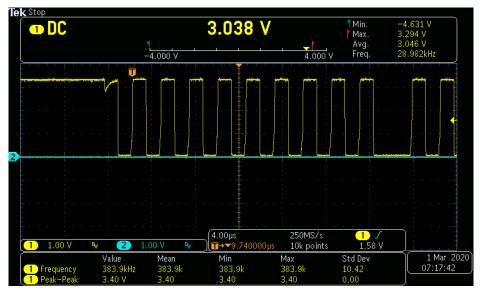
You can now achieve much faster data rates without having to noodle with resistors, and over long cables. We ran a 400 KHz OLED over 3 meters of phone wire with ease. With a 100KHz signal, we even ran a BME680 over 100 feet of Ethernet (about 3000pF round trip! (https://adafru.it/NDa)), and had an OLED display the sensor details.
