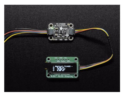
The TLV493D 3-axis magnetometer is a great little sensor for detecting magnets *in 3D*. (https://adafru.it/FN5) In fact, the manufacturer Infineon suggests it could be used to make a joystick! You could also use it for other cool things like detecting objects with magnets attached, like the lid of a box, or maybe a statue that unlocks your secret lair when placed on your mantle?
