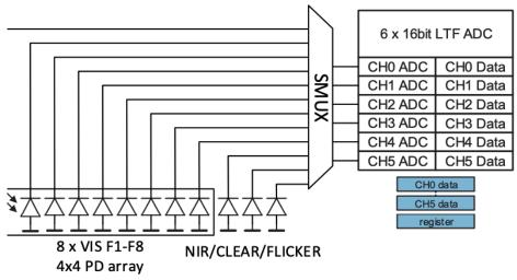
11 readable individual sensor elements (10 light channels plus flicker detection) don't exactly fit through a 6-channel ADC all at once, so the chip includes a so-called Super MUX (SMUX) that allows you to route the signal from any sensor to any ADC channel. Now that's some super multiplexing! The sensor also has GPIO and interrupt pins that can allow it to communicate directly with other sensors, or the microcontroller itself.
