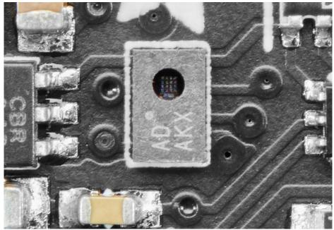
The super-human color measuring capabilities of the AS7341 can be used to quantify the specific makeup of whatever interesting colors you can point it at, and can do so with more accuracy and specificity than a
