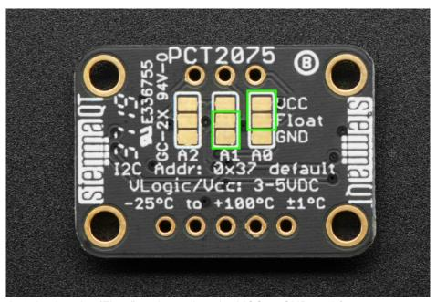
All you need to do is bridge the "Float" pad to either the VCC or GND pad for one or more of the address pins. In the picture above if you bridged the solder pads that are circled, you would pull A0 high to VCC and A1 low to GND. Referring to the table above this would set the address of the breakout to **0x72**
