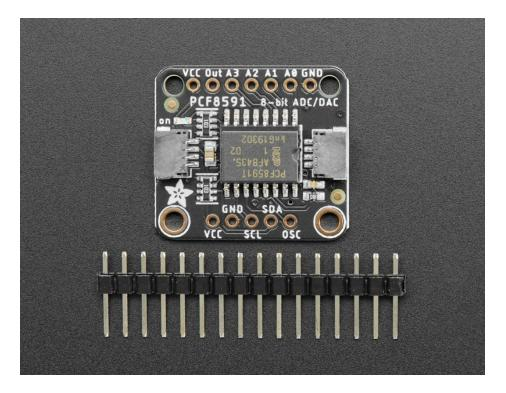
Along with four 8-bit ADC channels, the PCF8591 comes complete with an 8-bit **D**igital to **A**nalog **C**onverter converter as well! Not only can you measure voltages, but now you can *create* them just as you want them. You can even use the DAC and ADC together to create an input to a circuit and measure the results with the ADC. The possibilities abound!
