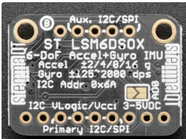
The backs of the breakouts show additional information about the specifications of the sensor, as well as the I2C address and additional pin information
