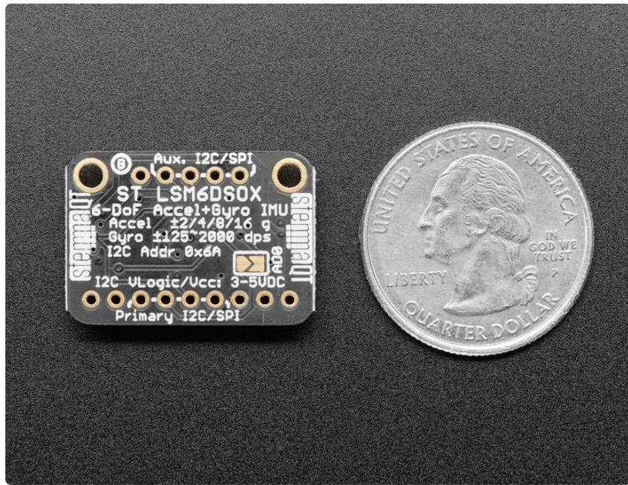
All three sensors are great IMU sensors with 6 degrees of freedom - 3 degrees each of linear acceleration and angular velocity at varying rates within a respectable range.
