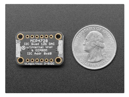
To take things even further, the MCP4728 lets you chose between two sources for your reference voltage: the input voltage that you use to power it on the VCC pin, or an **internal 2.048V reference voltage**. **If you**
