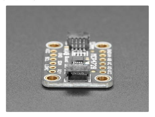
The breakout for the MCP4728 is populated with the required support circuitry to use it with your microcontroller of choice or Blinka-supported computer. The <a href="SparkFun Qwiic">SparkFun Qwiic</a> (https://adafru.it/Fpw) compatible <a href="STEMMA QT">STEMMA QT</a> (https://adafru.it/Ft4) JST SH connectors ease the process of connecting the MCP4728 to your project and allows you to easily share an I2C bus with other STEMMA QT, Qwiic, Grove or other compatible sensors.
