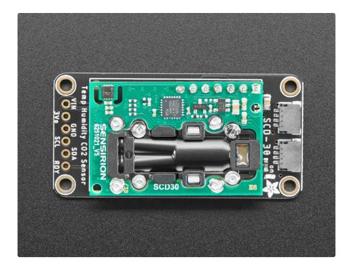
Data is read over I2C, so it works very nicely with just about any microcontroller or microcomputer. We've written both Arduino and Python/CircuitPython code so you can get started in a jiffy. Another nice element to this sensor is it comes with an <a href="https://started-in/shrtf">SHT31 temperature and humidity sensor already built</a> in (https://adafru.it/y7f). The sensor is used to compensate the NDIR CO2 sensor, but its also readable so you get full environmental data.
