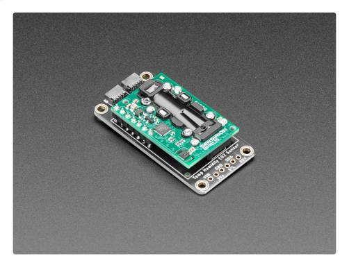
The SCD-30 is an NDIR sensor (https://adafru.it/CQ6), which is a 'true' CO2 sensor, that will tell you the CO2 PPM (parts-per-million) composition of ambient air. Unlike the SGP30, this sensor isn't approximating it from VOC gas concentration (https://adafru.it/PF7) - it really is measuring the CO2 concentration! That means its a lot bigger and more expensive, but it is the real thing. Perfect for environmental sensing, scientific experiments, air quality and ventilation studies and more.
