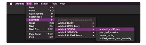
After opening the demo file, upload to your Arduino wired up to the sensor. Once you upload the code, you will see the **temperature**, **humidity and eCO2 data** values being printed when you open the Serial Monitor (**Tools->Serial Monitor**) at **115200 baud**, similar to this:
