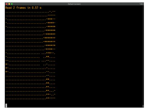
If you change the values for the variables at the top of the program, you can switch from printing out an ASCII image to printing out the temperatures in a grid. Change **PRINT\_TEMPERATURES** to **True** and **PRINT\_ASCIIART** to **False**, so that the two lines are as follows:
