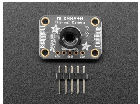
This sensor reads the data twice per frame, in a checker-board pattern, so it's normal to see a checkerboard dither effect when moving the sensor around - the effect isn't noticeable when things move slowly.
