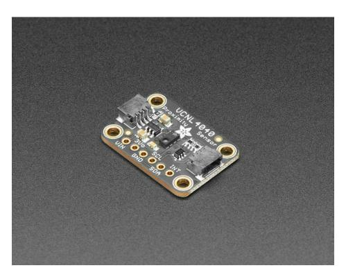
The VCNL4040 is a handy two-in-one sensor, with a proximity sensor that works from 0 to 200mm (about 7.5 inches) and light sensor with range of 0.0125 to 6553 lux.
