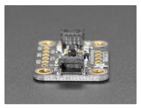
To make life easier so you can focus on your important work, we've taken the LIS3MDL and put it onto a breakout PCB along with support circuitry to let you use this little wonder with 3.3V (Feather/Raspberry Pi) or 5V (Arduino/ Metro328) logic levels.
