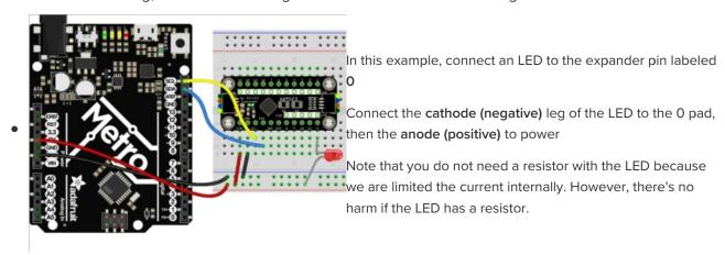
Constant current mode is open drain sink ONLY. That means you must connect LED negative sides to the pin and the positive sides to power - this is opposite from how we normally drive LEDs from a GPIO pin
