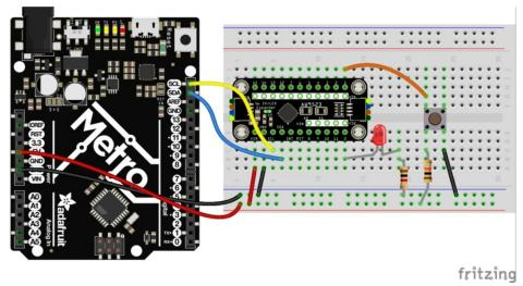
Open up File -> Examples -> Adafruit AW9523 -> ledbutton\_demo and upload to your Arduino wired up to the breakout.
