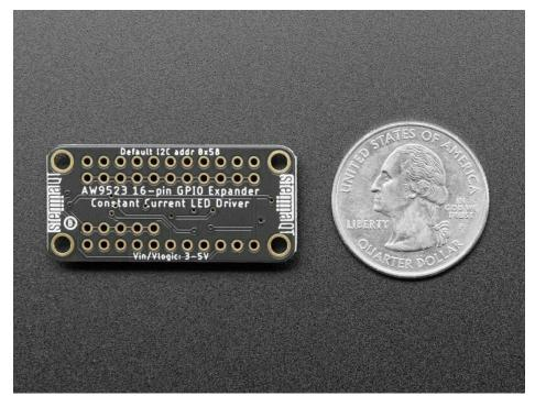
One oddity about this chip is the default I2C address determines the initial boot-state of the pins. Our
