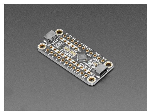
The lack of internally-configurable pull's is a bit of a bummer, but we think the expander more than makes up for it with the constant-current LED drive. If you're using an expander to add lots of controllable LEDs, this board will make it very easy. Since its constant-current, you *don't* need resistors in line with each LED (although it won't hurt if you do): simply connect the LED anode to one of the many VIN pads, then connect the cathode to the GPIO pin.
