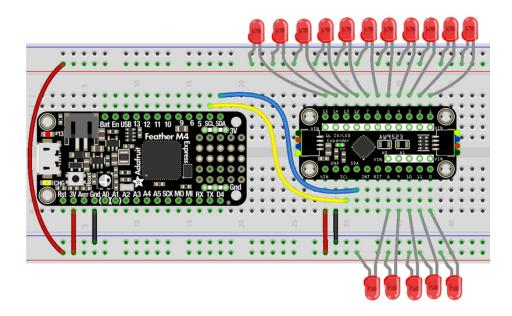
Constant current mode is open drain sink ONLY. That means you must connect LED negative sides to the pin and the positive sides to power - this is opposite from how we normally drive LEDs from a GPIO pin
