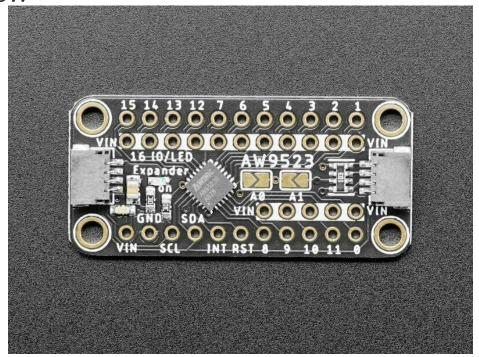
Expand your project possibilities, with the Adafruit AW9523 GPIO Expander and LED Driver Breakout - a cute and powerful I2C expander with a lot of tricks up it's sleeve.
