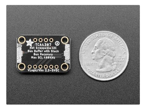
The chip can handle up to 400KHz I2C clock rates and even has stuck bus recovery: it automatically disconnects the bus if it detects either SDAOUT or SCLOUT are low for about 40 ms. Once the bus is disconnected, the device automatically generates up to 16 pulses on SCLOUT to attempt to reset the device which is holding the bus low.
