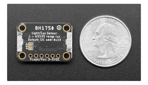
The BH1750 provides 16-bit light measurements in lux, the SI unit for measuring light making it easy to compare against other values like references and measurements from other sensors. Able to measure from 0 to 65K+ lux, the BH1750. With some calibration and advanced adjustment of the measurement time, it can even be convinced to measure as much as 100,000 lux!
