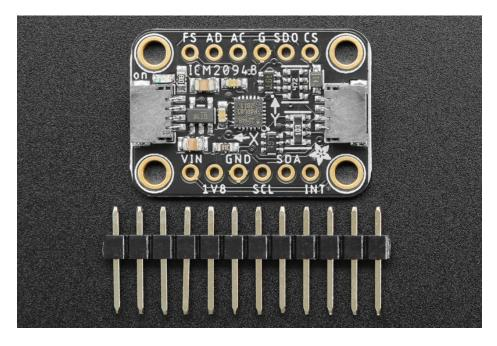
All 9 axes of measurement are made available thanks to a crew of 16-bit Analog to Digital Converters, diligently
