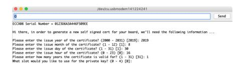
The issue date, expiration date, and signature are stored in a different slot on the ATECC608A. Select a slot to use for storing these values.
