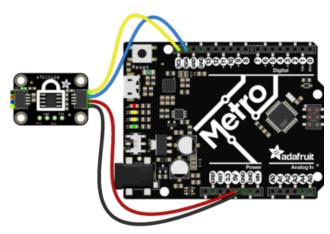
Connect Metro or Arduino 5V to board Vcc Connect Metro or Arduino GND to board GND Connect Metro or Arduino SDA to board SDA Connect Metro or Arduino SCL to board SCL
