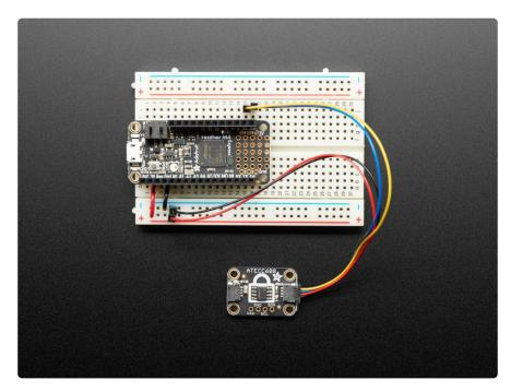
Please note the I2C address is fixed at 0x60 and according to Microchip, you should use this at higher I2C speeds like 400KHz if other devices are on the I2C bus, to avoid some I2C bus contention (much like the datasheet, this is not documented anywhere yet).
