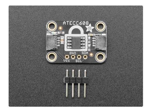
To make working with the ATECC608 as easy as possible, we've put it on a breakout PCB with the required support circuitry and <u>SparkFun qwiic</u> () compatible <u>STEMMA</u> <u>QT</u> () connectors. This allows you to use it with other similarly equipped boards withou t needing to solder. This chip will work with 3.3V or 5V power/logic micros, so it's ready to get to work with a range of development boards.
