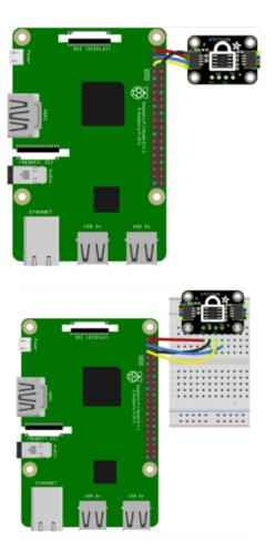
Pi 3V to sensor VIN (red wire) Pi GND to sensor GND (black wire) Pi SCL to sensor SCL (yellow wire) Pi SDA to sensor SDA (blue wire)
