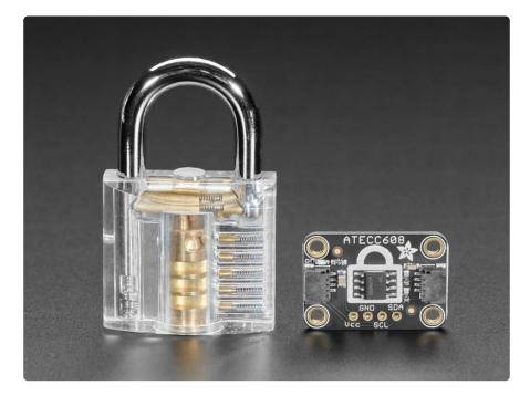
The ATECC608 is the latest crypto-auth chip from Microchip, and it uses I2C to send/ receive commands. Once you 'lock' the chip with your details, you can use it for ECDH and AES-128 encrypt/decrypt/signing. There's also hardware support for random number generation, and SHA-256/HMAC hash functions to greatly speed up a slower micro's cryptography commands.
