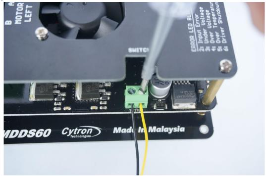
1) Connect Switch to the terminal block.
