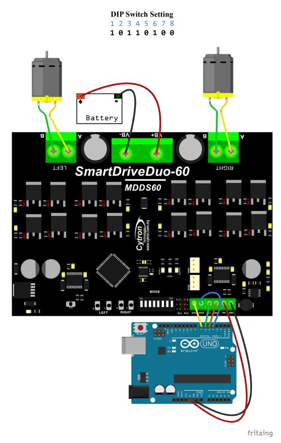
PWM input mode with microcontroller (Independent Both), DIP switch
