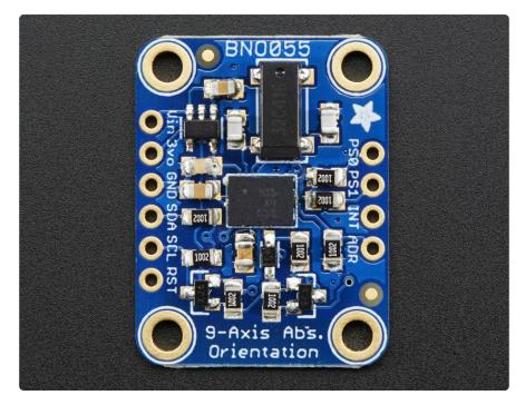
If you've ever ordered and wire up a 9-DOF sensor, chances are you've also realized the challenge of turning the sensor data from an accelerometer, gyroscope and magnetometer into actual "3D space orientation"! Orientation is a hard problem to solve. The sensor fusion algorithms (the secret sauce that blends accelerometer, magnetometer and gyroscope data into stable three-axis orientation output) can be mind-numbingly difficult to get right and implement on low cost real time systems.
