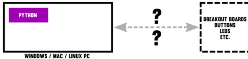
The MCP2221 provides another way to do this by utilizing the USB bus. The MCP2221 just makes different trade offs relative to the FT232H. The biggest being **no hardware SPI support**. But you do gain ADC and DAC support. Also, it's much cheaper than the FT232H.
