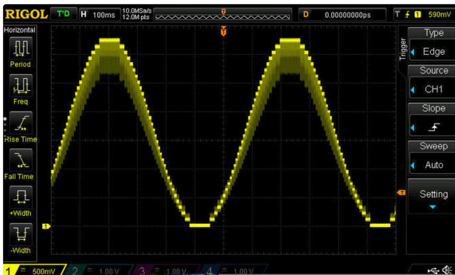
Note that even though the MCP221's DAC is only 5 bits, you set it using a 16 bit value to comply with the CircuitPython API.
