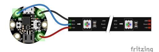
Note that the wire ordering on your NeoPixel strip or shape may not exactly match the diagram above. Check the markings to verify which pin is DIN, 5V and GND
