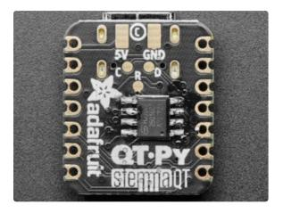
Once soldered in, you can access the SPI flash in Arduino on **SPI1** and chip select pin **17**. In CircuitPython, a 'haxpress' version of the runtime will need to be installed, so it knows to look for the larger filesystem. There is more hardware support in the haxpress CircuitPython build because we can add more code to the internal flash instead of using it for a filesystem
