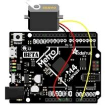
For the Metro M4 Express, ItsyBitsy M4 Express and the Feather M4 Express, connect the ground wire to any G or GND, the power wire to USB or 5V, and the signal wire to A1.
