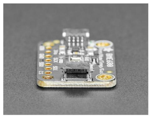
To make things easier and a bit more flexible, we've also included SparkFun Qwiic (https://adafru.it/Fpw) compatible STEMMA QT (https://adafru.it/Ft4) connectors for the I2C bus so you don't even need to solder! Just plug in a compatible cable and attach it to your MCU of choice, and you're ready to load up some software and measure some light.
