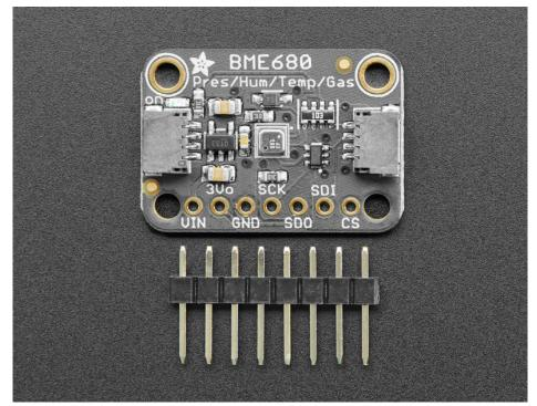
The BME680 takes those sensors to the next step in that it contains a small MOX sensor. The heated metal oxide changes resistance based on the volatile organic compounds (VOC) in the air, so it can be used to detect gasses & alcohols such as Ethanol, Alcohol and Carbon Monoxide and perform air quality measurements. Note it will give you one resistance value, with overall VOC content, it cannot differentiate gasses or alcohols.
