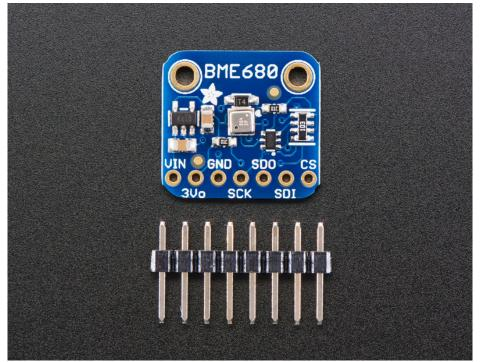
For your convenience we've pick-and-placed the sensor on a PCB with a 3.3V regulator and some level shifting so it can be easily used with your favorite 3.3V or 5V microcontroller.
