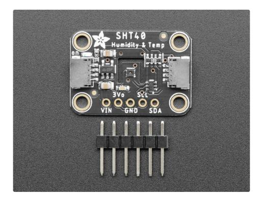
If you prefer working on a breadboard, each order comes with one fully assembled and tested PCB breakout and a small piece of header. You'll need to solder the header onto the PCB, but it's fairly easy and takes only a few minutes even for a beginner.
