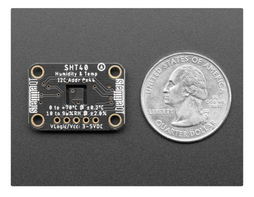
Unlike some earlier SHT sensors, this sensor has a *true* I2C interface for easy interfacing with only two wires (plus power and ground!). Thanks to the voltage regulator and level shifting circuitry we've included on the breakout It is also is 3V or 5V compliant, so you can power and communicate with it using any microcontroller or microcomputer.
