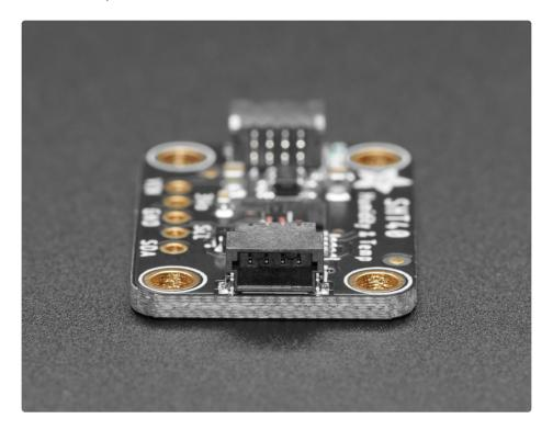
Such a lovely chip - so we spun up a breakout board with the SHT4x and some supporting circuitry such as pullup resistors and capacitors. To make things even easier, we've included <a href="SparkFun">SparkFun</a>
