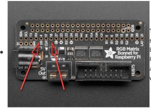
The "quality" option comes at a cost. First, you need to solder a jumper wire between GPIO4 and GPIO18 on the Bonnet or Hat board. Also, the normal sound output of the Raspberry Pi must be disabled. You can still use a USB sound adapter if needed, but audio over HDMI or from the 1/8" jack will not be present.
