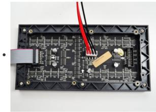
IDC goes into the INPUT side (look for any arrows, arrows point from INPUT side to OUTPUT)
