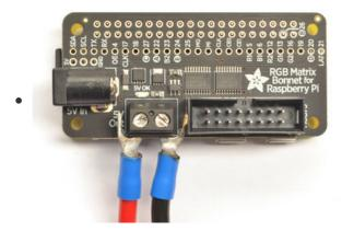
Plug the red wire into the + side, and the black wire into the - side.
