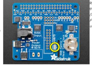
If you're using a 64x64 RGB matrix and either a Bonnet or a Rev C HAT, use your soldering iron to melt a blob of solder on the bottom solder jumper so the middle pad is 'shorted' to 8. (This is compatible with 64x64 matrices in the Adafruit store. For 64x64 matrices from other sources, you might need to use 16 instead, check the datasheet.)
