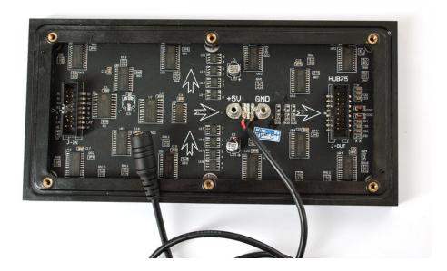
If your panel has the Molex-style header, just plug in the included power cable, observing the correct polarity.
