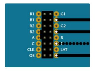
**32x32** and **64x32** matrices require **three** ground connections. **32x16** matrices have **four**.
