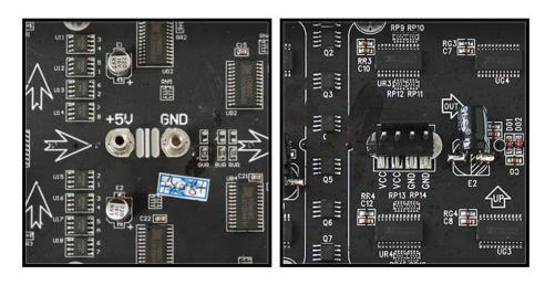
On the left is a screw post power connector (with adjacent pads for soldering wires directly). On the right, a Molex-style header. Some panels will have *two* headers...the power cable included with these panels has connectors for both headers.
