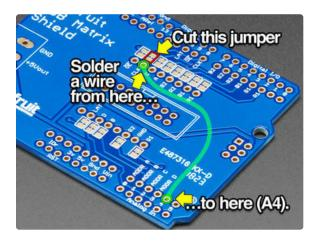
The shield requires a small modification to work with the Adafruit **Metro M4**:
