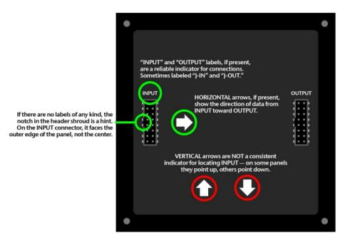
The arrangement of pins on the INPUT connector varies with matrix size and the batch in which it was
