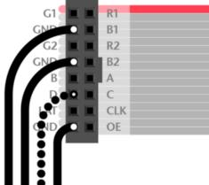
**32x32** and **64x32** matrices require **three** ground connections. **32x16** matrices have **four**.
