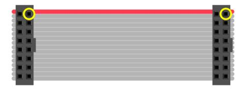
Either end of the ribbon cable can be plugged into the matrix INPUT socket.
