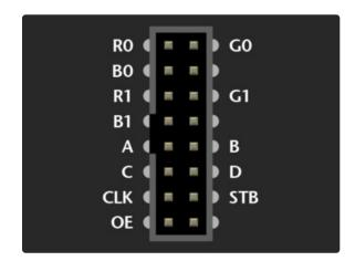
A **32x16** panel uses this pin arrangement. The labels might be slightly different, or the pins might not be labeled at all...but in either case, use this image for reference.
