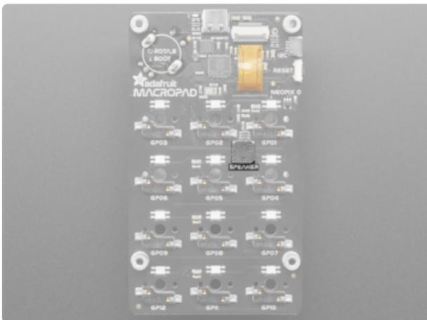
The grey square a bit to the right of the center of the board on the back is the 8mm speaker/buzzer. With a Class D amplifier and RC filter, it can be used to make simple beeps and sounds effects.
