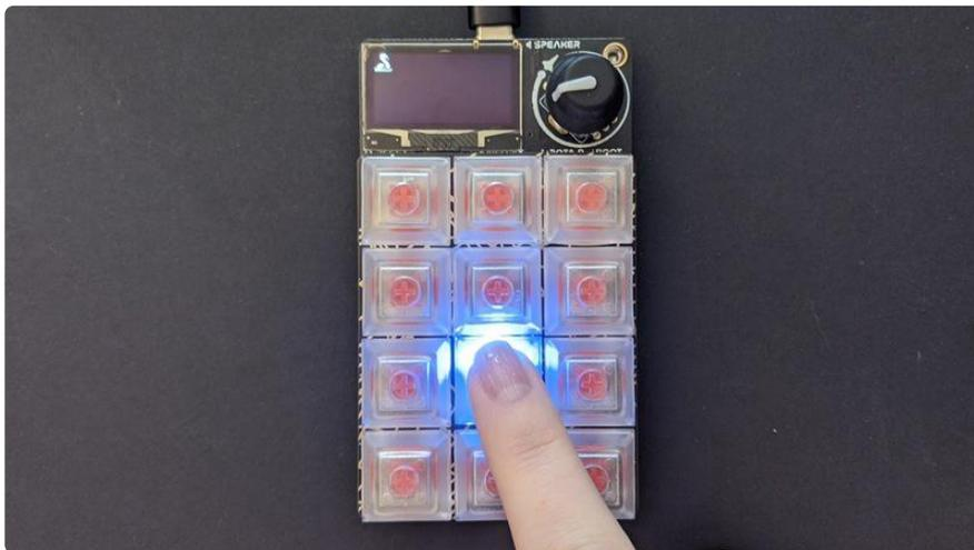
The MacroPad library includes the ability to play tones, either for a specified duration, for example, 0.5 seconds, or until you tell it to stop in your code, for example, the duration of a key press.
