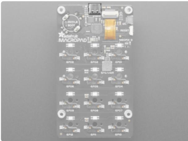
At the top-center of the board, visible from both sides, is the USB Type C connector. This connector is used both for transferring data from your computer (e.g. updating your CircuitPython code.py file, or uploading an Arduino sketch) and powering the board.
