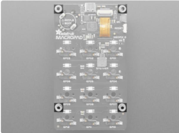
Arranged in the top two corners of the board, and towards the bottom two corners are four mounting bosses to allow for using the [MacroPad enclosure kit](https://adafru.it/TAE) or designing your own enclosures.
