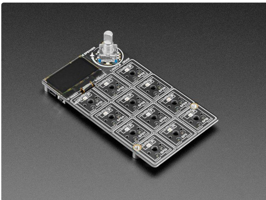
Get ready to upgrade your desk's mission control station with a CircuitPython or Arduino powered Macropad - complete with 12 buttons, OLED display, speaker and rotary encoder. Customize it for your spacecraft to help guide you through the great reaches of the unknown. (Or just have it type out your favorite emojis.)
