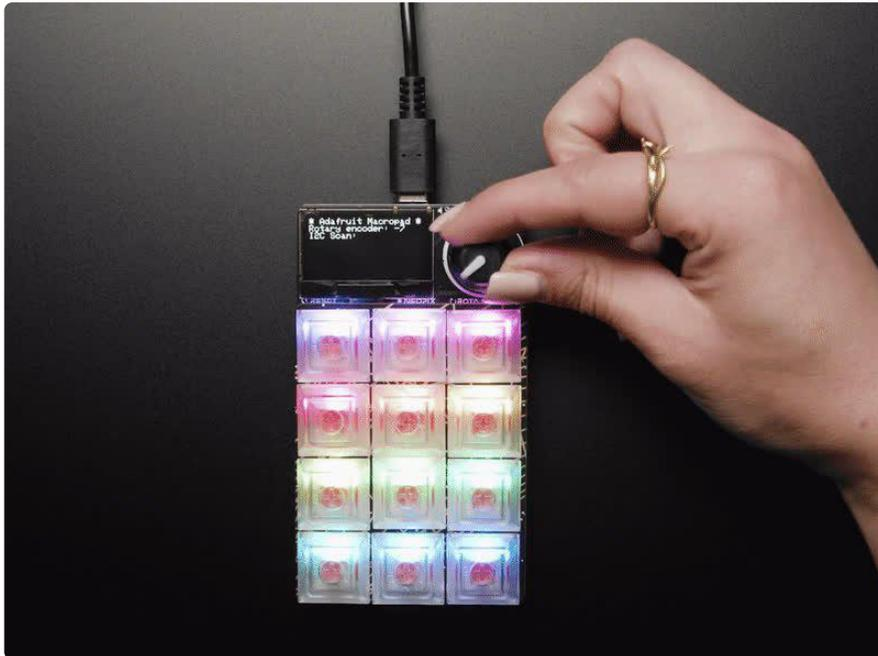
Strap yourself in, we're launching in T-minus 10 seconds...Destination? A new Class M planet called MACROPAD! M here, stands for Microcontroller because this 3x4 keyboard controller features the newest technology from the Raspberry Pi sector: say hello to the RP2040. It's speedy little microcontroller with lots of GPIO pins and a 64 times more RAM than the Apollo Guidance Computer. We added 8 MB of flash memory for plenty of storage.
