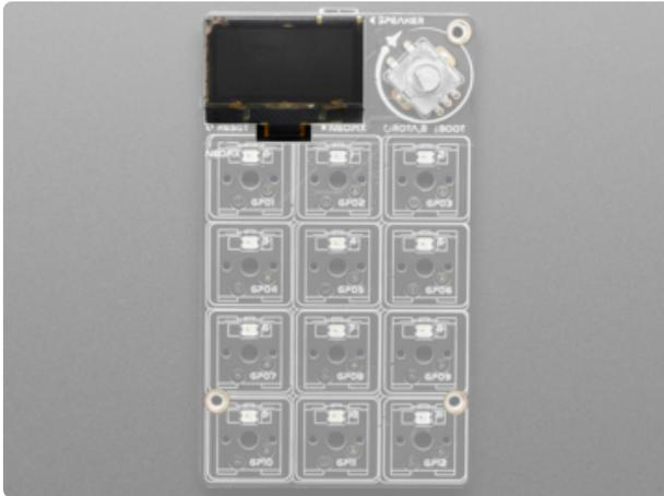
On the top left corner of the board (when viewed from the top), is the 128x64 SH1106 Monochrome OLED display. The ribbon cable for the display goes through a hole in the board to the back, where it is inserted into the display connector. This OLED is on high-speed hardware SPI to ensure quick updates.
