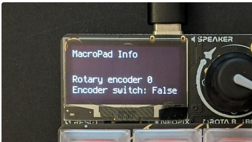
If you rotate the rotary encoder, the number will change. It doesn't matter where the rotary encoder is, it will begin at 0. The number provided is a relative position.
