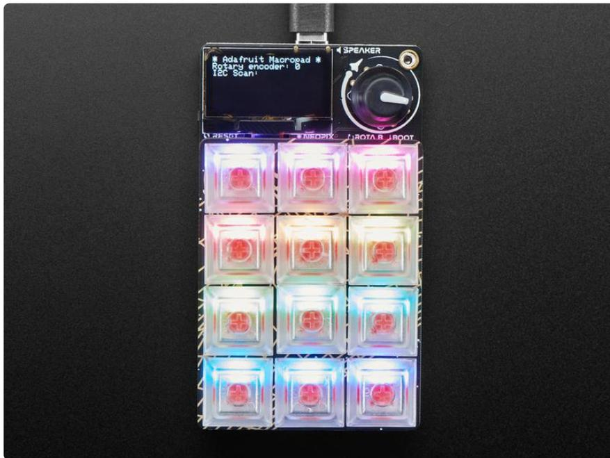
This space-ship is also fitted with a 128x64 monochrome OLED for a crisp heads-up display that can be used in Arduino or CircuitPython to display keymaps, stats, computer performance, etc. There's also a rotary encoder with push-button soldered in. Twist and turn it or push to change volume or monitor brightness or scroll: whatever you like! A tiny speaker can give audio feedback or play fun bleepy tunes.
