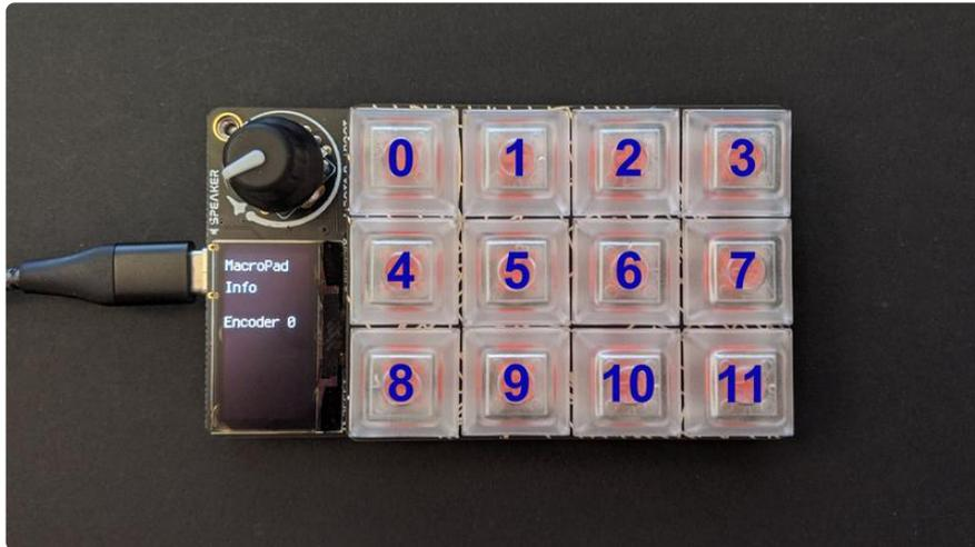
This example rotates the MacroPad 90 degrees. Remember, when the MacroPad is in a sideways orientation, the display is 64x128 pixels (instead of the standard 128x64 pixels). Any text displayed needs to be shortened to fit on the display. So, this example puts the title on two lines to shorten it up and uses shorter strings than [the Display Text example \(https://adafru.it/Uat\)](https://adafru.it/Uat).
