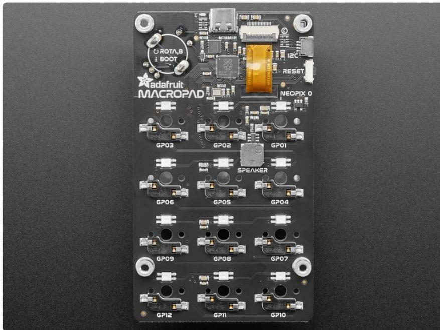
Please note, the RP2040 chip does not currently have QMK support - this macropad is designed to be programmed in Arduino or CircuitPython! If QMK eventually does add RP2040 as a supported chipset (no ETA and no plans that we know of), we'll update this page.
