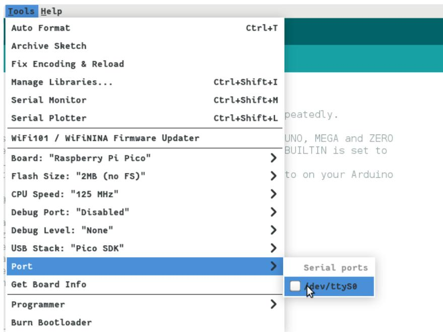
Note that after you flash your first sketch, the board will not show up as a USB drive and will use ports such as /dev/ttyACM0, COM, or /dev/tty.usbmodem14301. Make sure to change the port in Tools -> Port.
