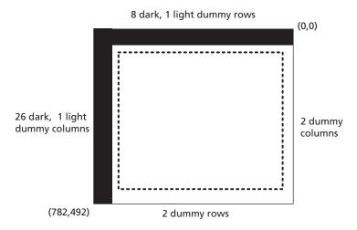
Figure 5: Pixel Color Pattern Detail (Top Right Corner)
