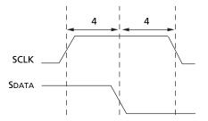
Figure 38: Serial Host Interface Stop Condition Timing
