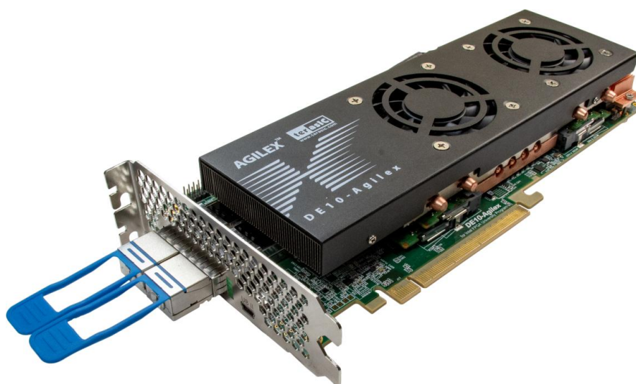
Figure 9-2 QSPF-DD Transceiver Loopback Test in Progress
